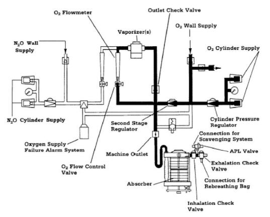
Oxygen and  $N_2O$  flow from cylinders and or wall outlet though flowmeters, along the backbar, though calibrated vaporiser and then via the machine common gas outlet to the breathing system. (Reproduced by permission of Datex-Ohmeda).
